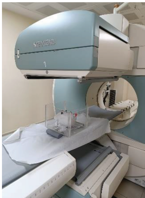
Figure 2. Position of the liver phantom in the SPECT/CT device within the water tank
