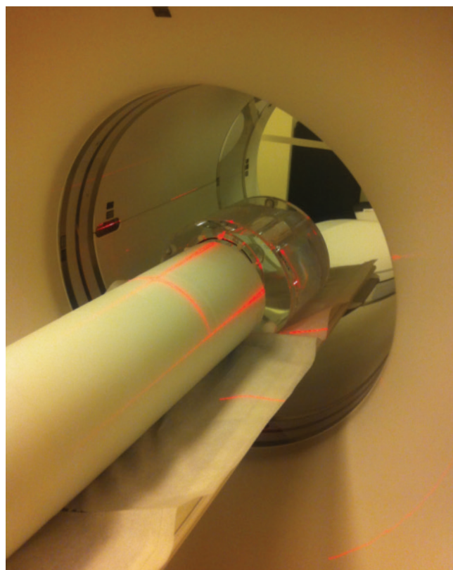
Figure 5. Positioning of polyethylene and body phantom
